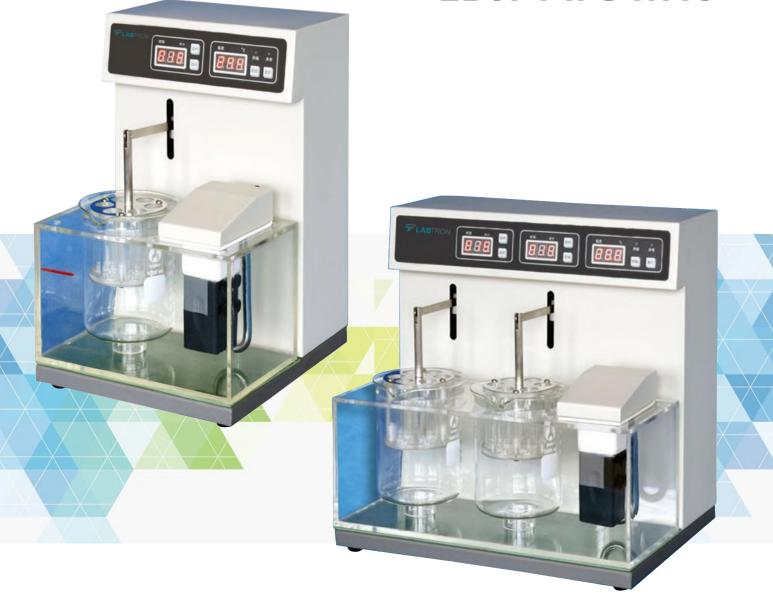
Disintegration tester LDIT-A1O is adopted with high-precision digital electronic sensor, ensures quality precision and accuracy of the water bath temperature without need for calibration. Equipped with one set of basket to conduct disintegration experiments. The default setting for lifting time of the basket is 15 mins, can manually set the other time value as per the experimental need.
