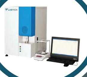
IR Carbon and Sulphur Analyzer
